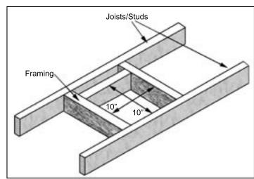
Figure 24. Vent Framing Through Wall/Ceiling
